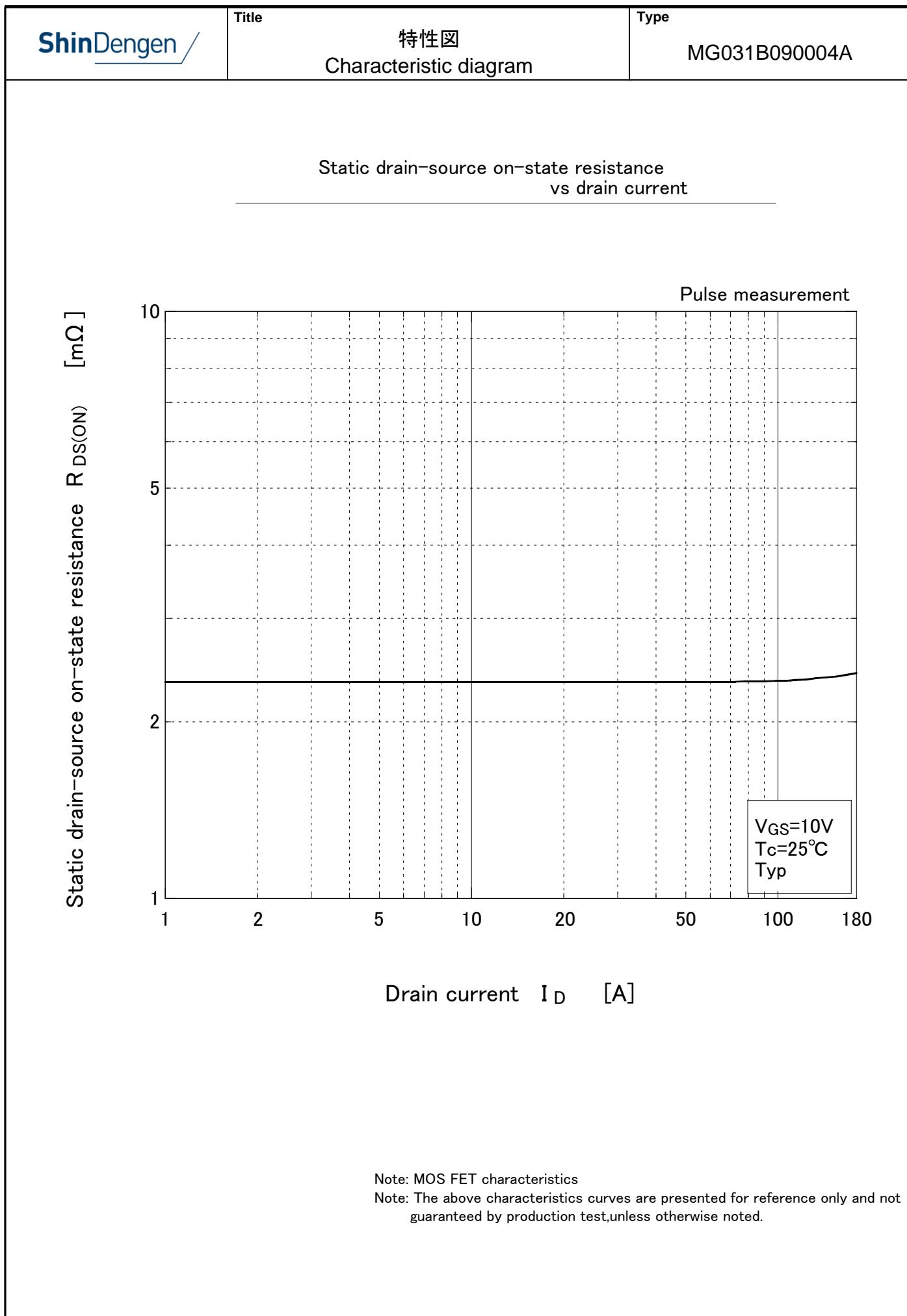
Static drain-source on-state resistance
