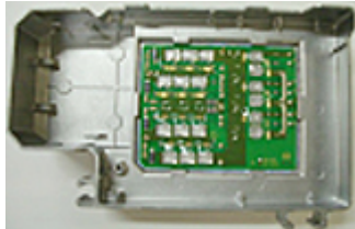
Power module section of sine wave inverter
